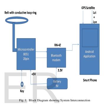
The 20 pin 8051 Microcontroller used has high performance & low power consumption device. The RN-42 Bluetooth modem has Low power sleep mode, perfect for short range(its range is about 50 to 60 feet ).
