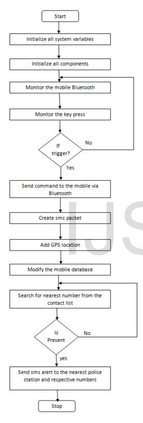
Fig. 2. System Flow Diagram
